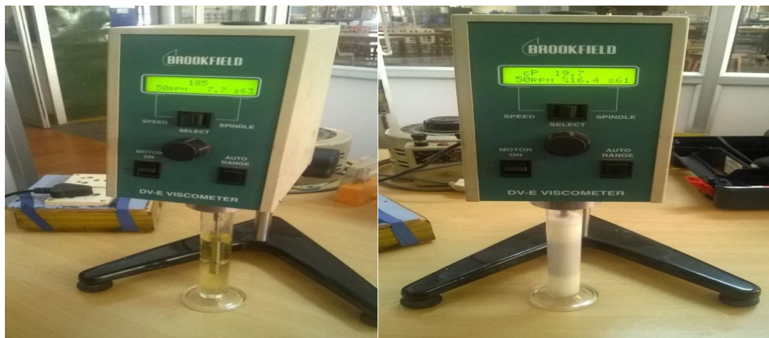
Fig1: Measurement of viscosity using viscometer with formulated oil and emulsion
