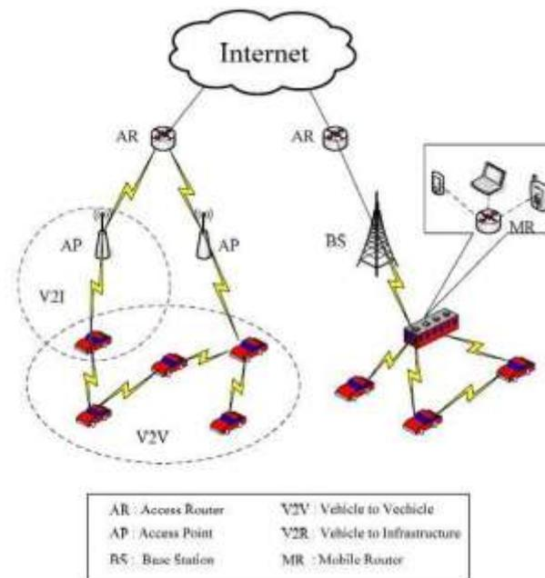
**Fig 2: General Model of Vehicular Networks**
