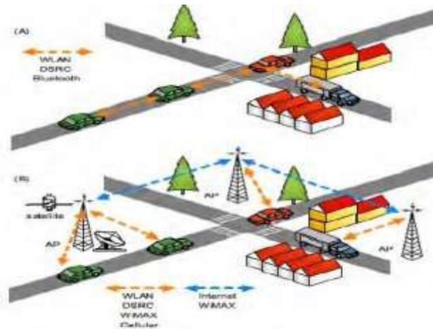
**Fig 1: Two types of Communication Modes of VANET : (a) V2V Communication (b) V2I Communication**
