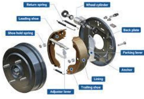
Fig.5. Drum Brake
