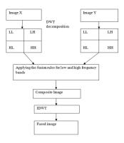
Fig. 2 Wavelet transform based fusion algorithm
