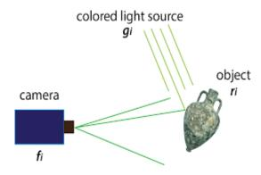
Fig. 1 Process of image capturing
