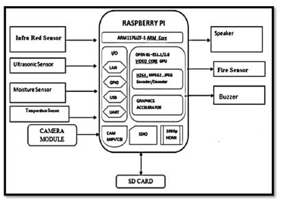
Fig.1. Block diagram of blind stick
