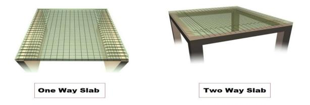
Figure 1: One Way and Two Way Slabs [8]
