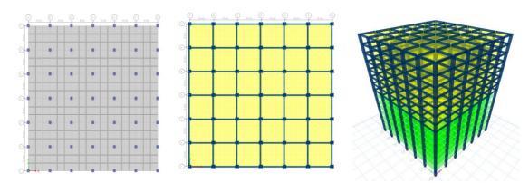
Figure 6: a. Plan view from Ground storey to 7<sup>th</sup> storey, b. Plan view from 8<sup>th</sup> storey to 15<sup>th</sup> storey and c. Elevation view of model GS+CS
