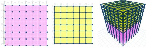
Figure 5: a. Plan view from Ground storey to 7<sup>th</sup> storey, b. Plan view from 8<sup>th</sup> storey to 15<sup>th</sup> storey and c. Elevation view of model FS+CS
