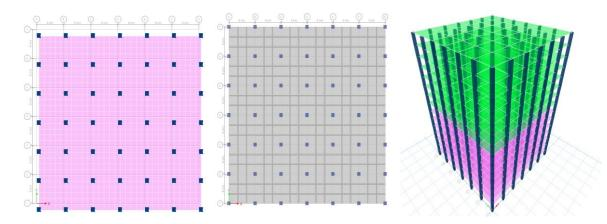
Figure 12: a. Plan view from Ground storey to 7<sup>th</sup> storey, b. Plan view from 8<sup>th</sup> storey to 15<sup>th</sup> storey and c. Elevation view of model FS+GS
