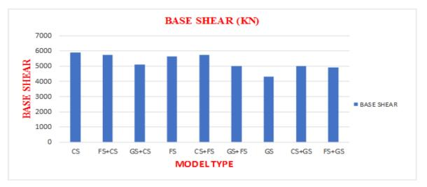
Figure 14: Base shears of RC Slab Systems for Zone V
