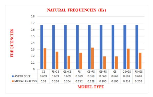
Figure 13: Comparison of Natural Frequencies of different RC Slab Systems with IS Code
