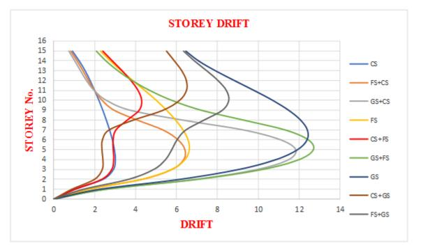
Figure 16: Storey Drifts of RC Slab Systems for Zone V
