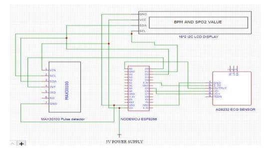
**Figure 4- CIRCUIT DIAGRAM**
