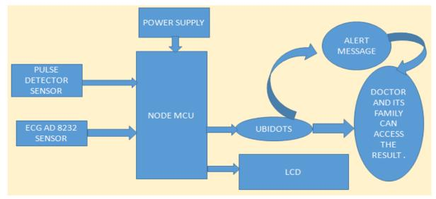
Figure 3- PROPOSED BLOCK DIAGRAM OF HEALTH MONITORING SYSTEM
