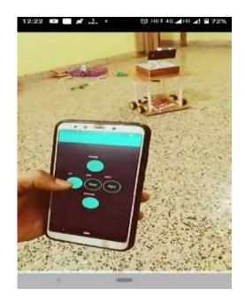
Fig5. The smart phone loaded with droid cam app streams the current situation of the ward by means of video streaming that could be seen at remote server
