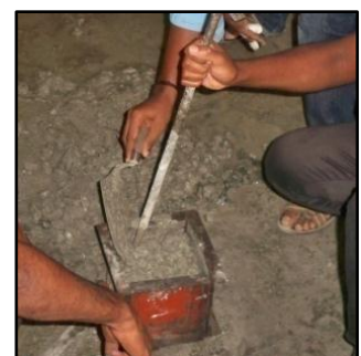
Fig 4: Casting the mix
