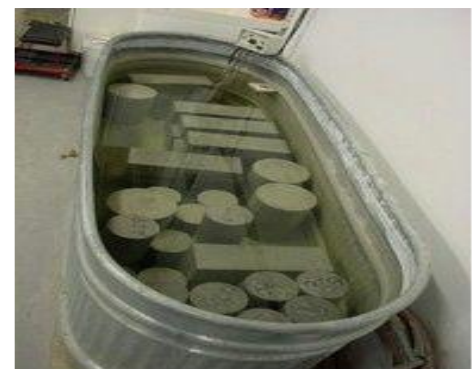
Fig 6: Curing the Specimen
