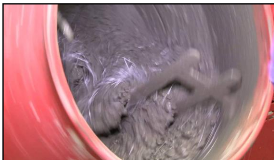
Fig 2 Mixing the fiber with concrete
