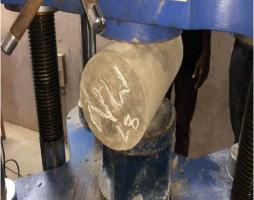
Split tensile strength of concrete is usually found by testing plain concrete cylinders. Cylinders of size 150mm x 300 mm were used to determine the split tensile strength. After curing, the specimens were tested for split tensile strength using the details of same are represented in table4.
