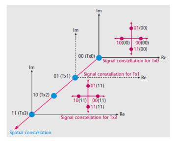
Figure 1. Tri-dimensional constellation diagram of SM
