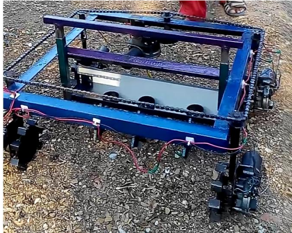
Figure 8.2 Fabricated model of Universal Seed Sowing Machine
