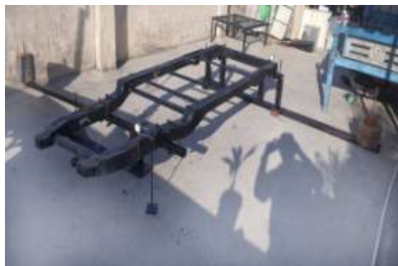
Fig.14 Actual model of torsional test rig.
