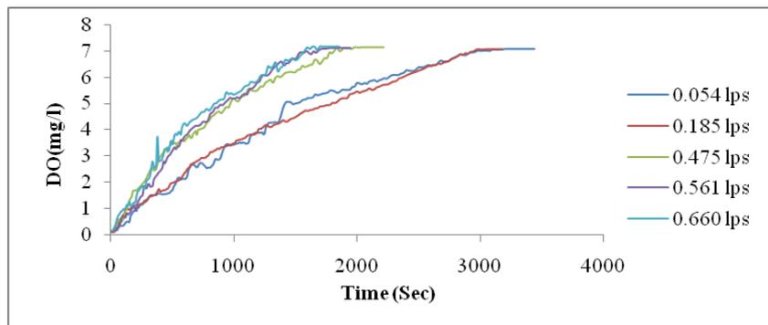
Figure 6: Variation of DO at different discharge for hole 2' of 5 mm effective length
