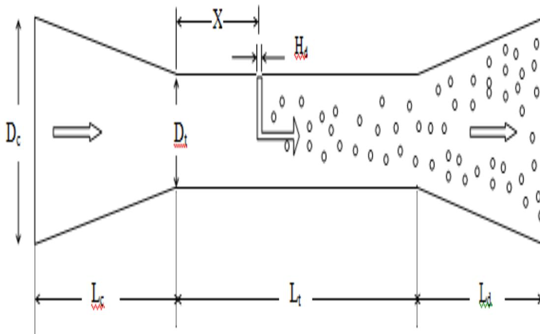
figure1: Geometric Parameters of the fabricated venture table : Details of the Venturi detail
