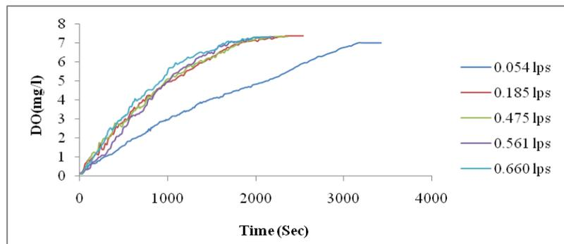
Figure 5: Variation of DO at different discharge for hole 1' of 2 mm effective length
