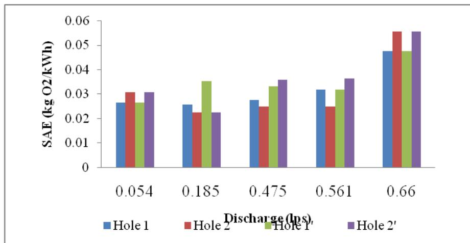
Figure 8: Effect of SAE with respect to the different discharge rates
