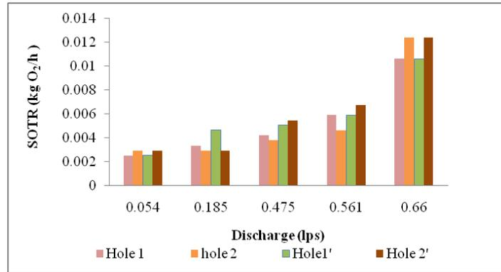
Figure 7: Effect of SOTR with respect to the different discharge rates
