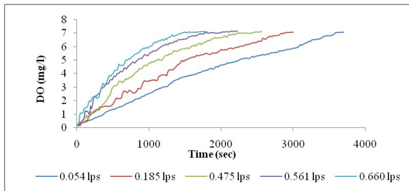
Figure 3: Variation of DO at different discharge for hole 1 of 3 mm effective length
