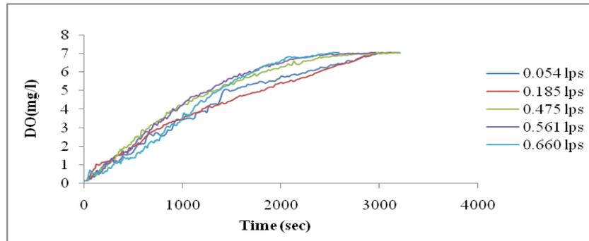
Figure 4: Variation of DO at different discharge for hole 2 of 7 mm effective length
