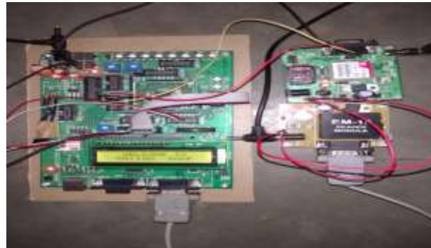
Fig. 5 Interfacing of RFID and GSM
