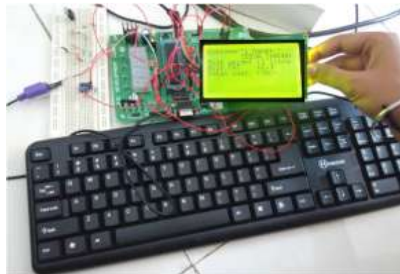
Fig. 4 Interfacing keyboard and GLCD with PIC
