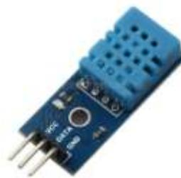
Fig 3: Humidity Sensor Module
