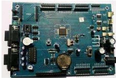
Fig 2: ARM LPC2148 microcontroller unit.
