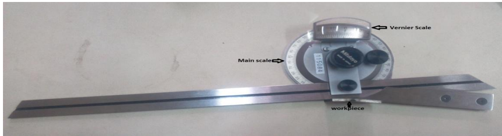
Fig5. Bevel protractor for measuring bending angles
