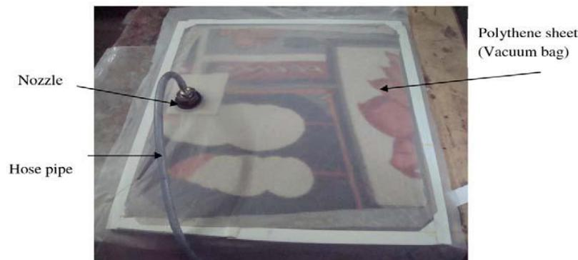
**Fig.1 Vacuum bagging process for manufacture of GFRP and GFRP mixed with Carbon Nanotubes**
