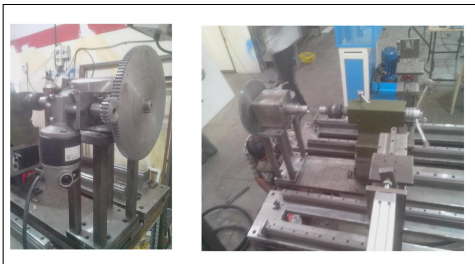
Fig.4.1 Assembly of Head Stock and Tail Stock
