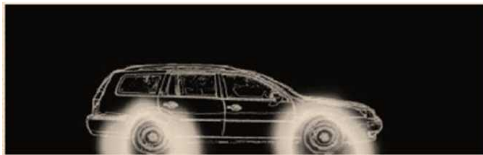
Fig. 2 Propagation of tyre noise of an automobile at frequency of 600Hz.
