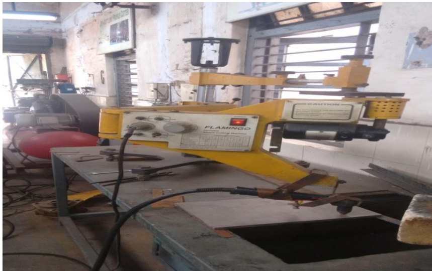
Fig. 3: Experimental setup used for the present study: An automatic profile cutter
