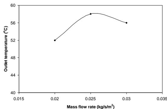
**Figure 5.1 Variation of outlet air temperature with air flow rate**
