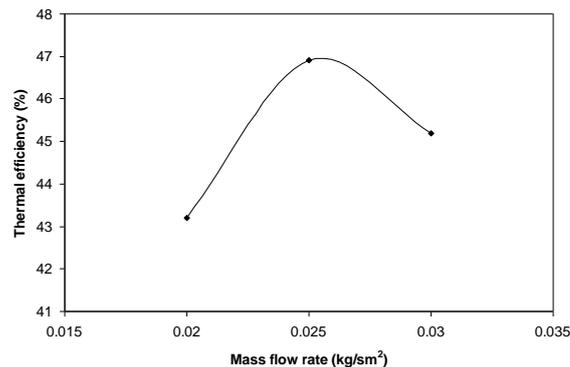
**Figure 5.2 Variation of thermal efficiency with air flow rate**
