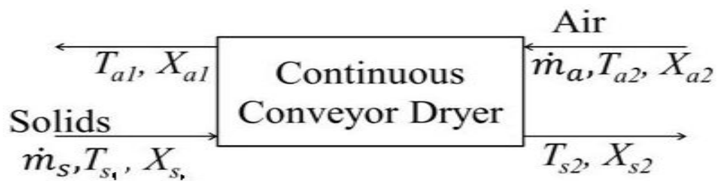
Fig-3- Flow Diagram for a Counter-Current Continuous Dryer
