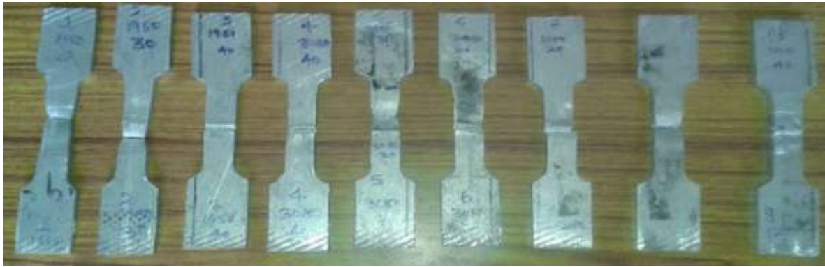
Fig. 6: The welded Al 1050 H8 Specimen After Tensile Test
