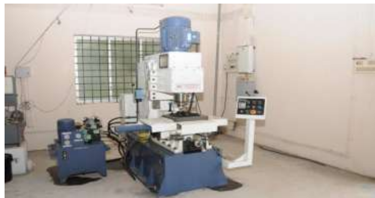
Fig. 2: The Experimental Setup of the Semi Automatic Friction Stir Welding Machine
