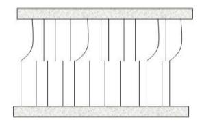
Figure 4: Concept of Bristles used in Lugre Model
