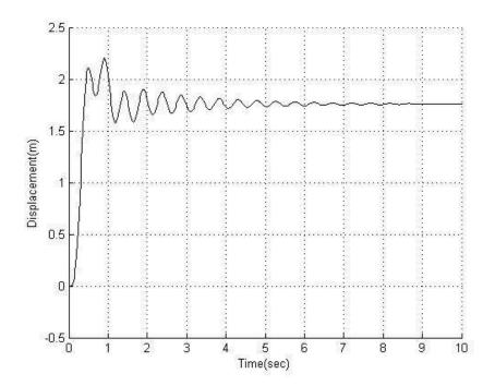
Figure 5: Dynamic Response or Hydraulic Actuator
