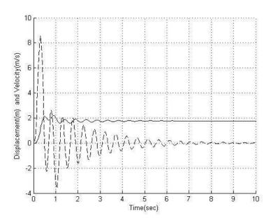
Figure 6: Dynamic Response or Hydraulic Actuator
