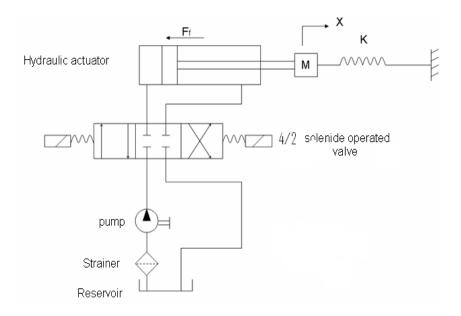
Figure 1: The Hydraulic System and Hydraulic Actuator
