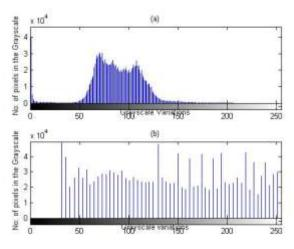
Figure 4: a) Histogram of the grayscale image, b) Equalized histogram of 5 a).
