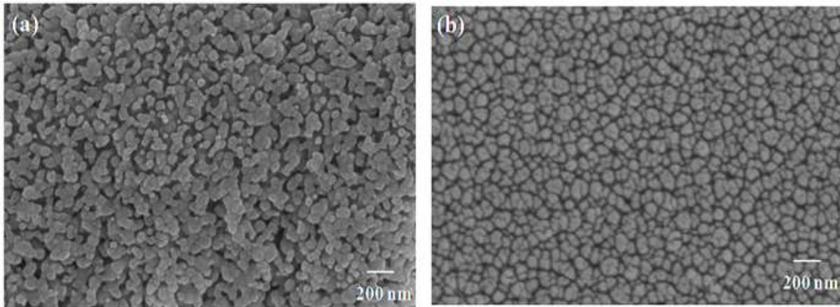
**Fig. 2: FESEM Image Of ZnO Thin Films Grown By Sol-Gel Spin Coating Method On Quartz Substrates Using Various Sol Concentrations (A) 0.6M And (B) 0.4M**
