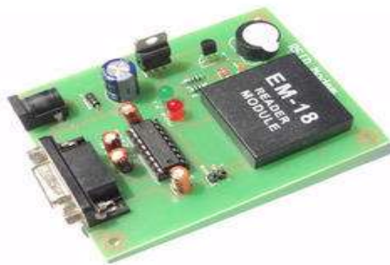
Fig 2(a): RFID reader
