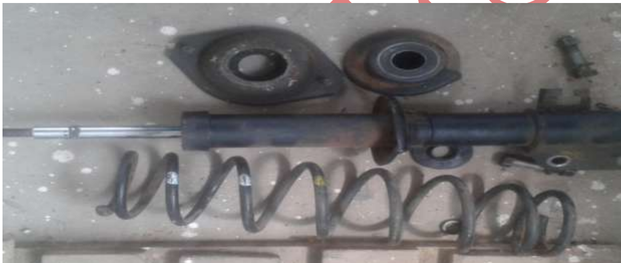
Image of Disassembled Suspension of a Car [MC Pherson]
