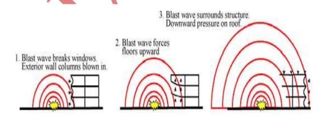
The initial shock wave is reflected and amplified by the ground surface to produce a reflected wave unlike the air burst, the reflected wave merges with the incident wave at the point of detonation and forms a single wave. In the majority of cases, terrorist activity occurs in built-up areas of cities, where devices are placed on or very near the ground surface.
