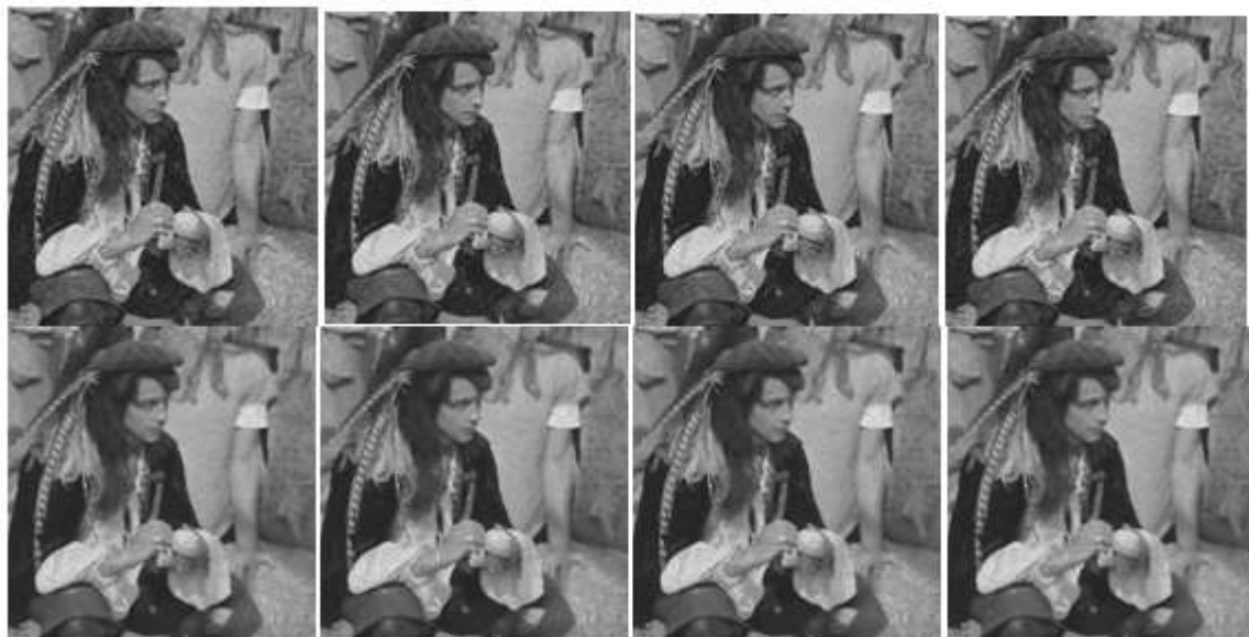
Fig 5 The First Row: Pirate Image With Speckle Noise With Noise Density Level D = 0.02, 0.04, 0.06, 0.08 ; Second Row: Corresponding Results Of Bilateral Filter
