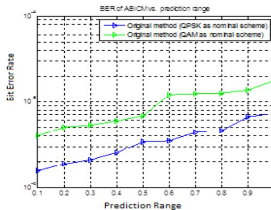
**Fig: 1 BER of ABICM vs. prediction range For the Rician Fading Channel**
