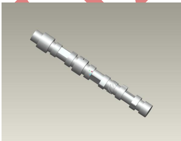
Fig. 5 Model of Camshaft Made In Pro-E Wildfire 4.0
