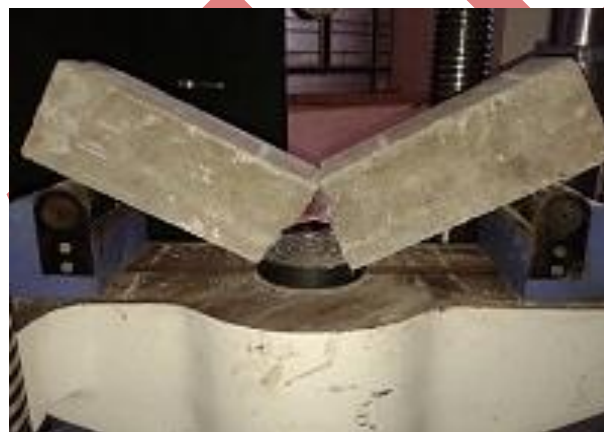
Fig: 10. Failure of beam without Reinforcement
