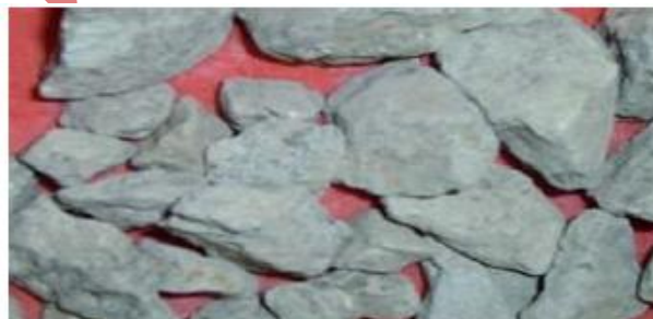
FIG 1:Coarse aggregate segregated from concrete waste
