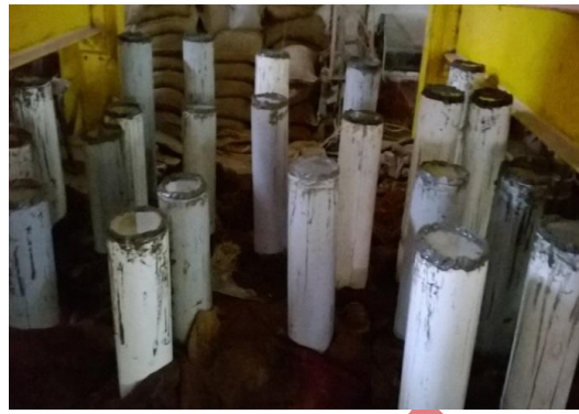
Fig 5: Water Curing by Ponding at the Top and Gunny Bags at the Bottom of Specimen
