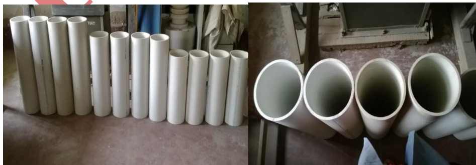
Fig 3: ASTM-D 1785 UPVC tubes of length 500, 600, 700mm having 150mm diameter
