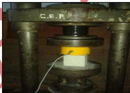
Fig.no.1 Rock samples with sensor mounting
