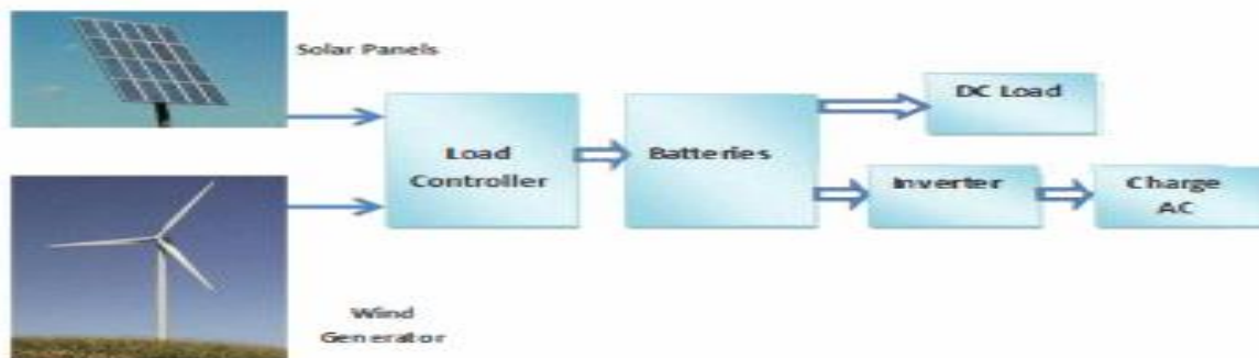
Figure (1): Off-grid solar-wind hybrid system
