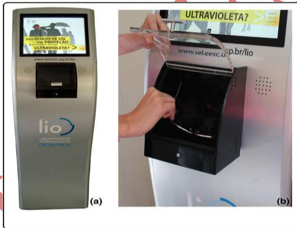
Figure 5 Picture of the available system for the public. (a) The self-service sunglasses testing kiosk; (b); inserting sunglasses for testing.
